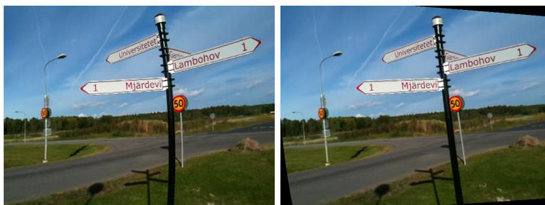
Figure 1: Image acquired during camera rotation on a rolling shutter cell-phone. Left: Video frame from iPhone3GS. Right: Rectification from our CVPR10 algorithm.
