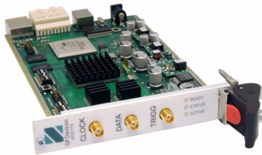
Figure 2. A data acquisition board utilizing principles for error correction developed during the CENIIT project. The board is the state-of-the-art for 14-bit resolution A/D-conversion supporting a sampling frequency of 840 MSps.
